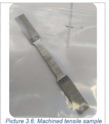
Picture 3.6: Machined tensile sample
